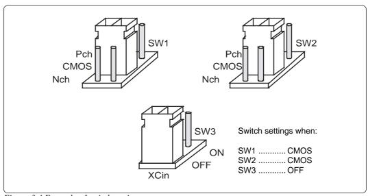
Figure 3.4 Example of switch settings
